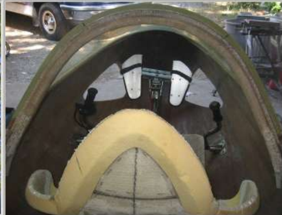
Pilot has view ports for enhanced underwater visibility
