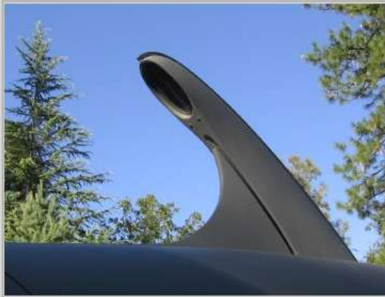
Snorkel valve automatically closes during dives
