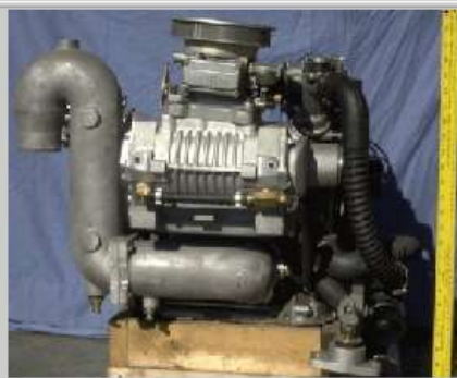
Supercharged rotary engine option generates over 250 hp!
