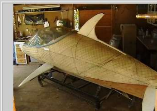
Body was constructed with fiberglass over PVC honeycomb
