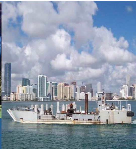
With the completion of columns the first phase was set in place with delivery to the projects "Little Mo" LCU. The total weight of the base and columns that had to be moved to the project site was over 2,000 tons.
